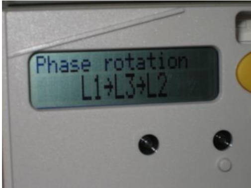
Figure 1 – Non-Standard Phase Rotation via Settlement Meter display.
